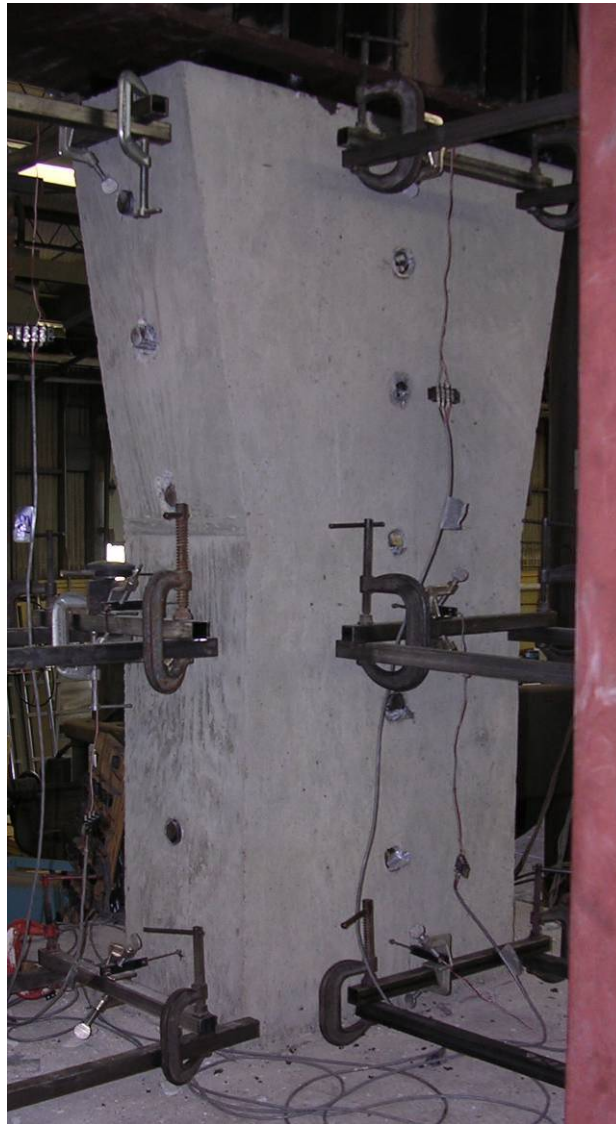
Figure 3.1: Control Column Ready for Testing
