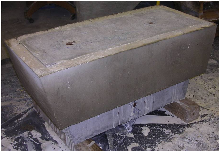
Figure 4.19: Concrete Jacket Repair
