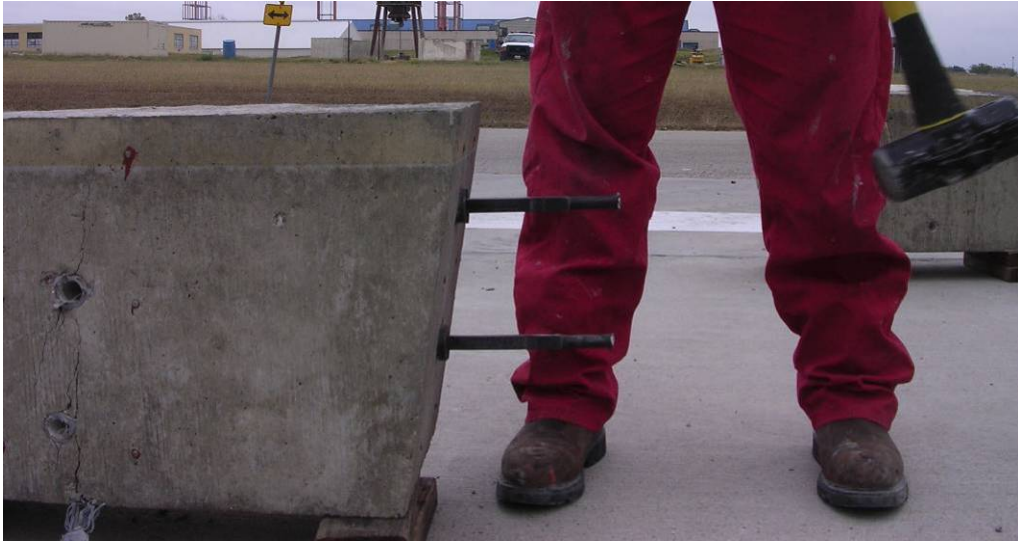
Figure 4.14: Splitting Wedges in Use to Damage Specimens
