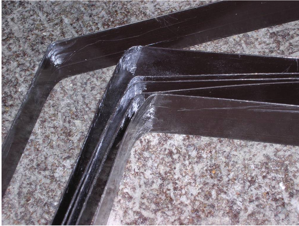
Figure 7.48: Packing Strap Corner Damage from Packing Strap #1
