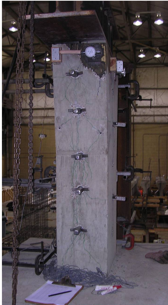
Figure 3.3: Mechanically Induced Cracking (Cracks Marked in Green)
