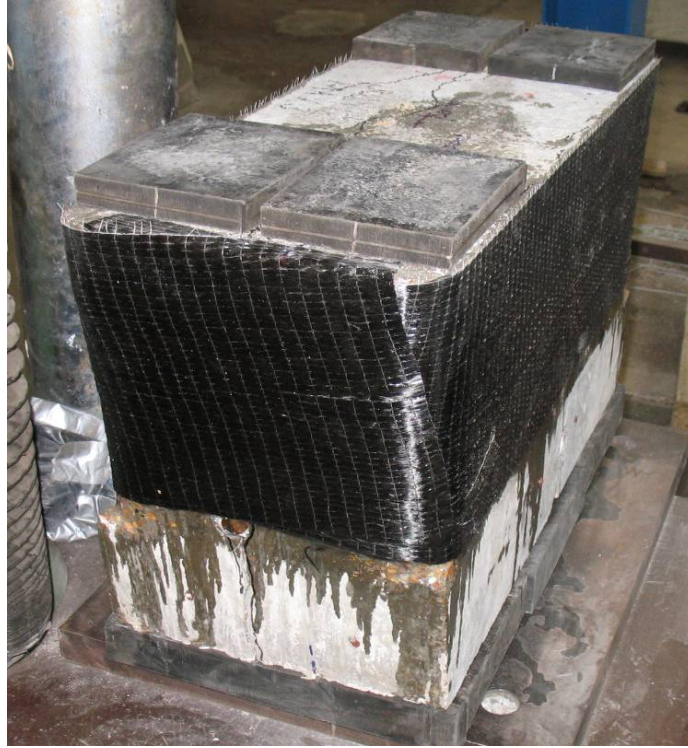
Figure 7.59: FRP #2 Specimen Prior to Testing
