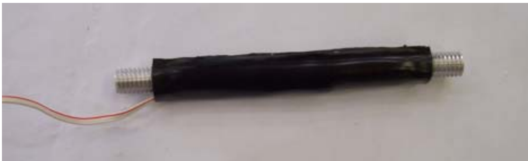
Figure A.11: Fifth, Wrap in Four-Inch Wide Mastic Tape (Barrier E)
