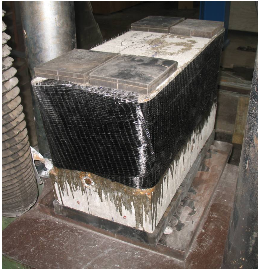
Figure 7.50: FRP #1 Specimen Prior to Testing
