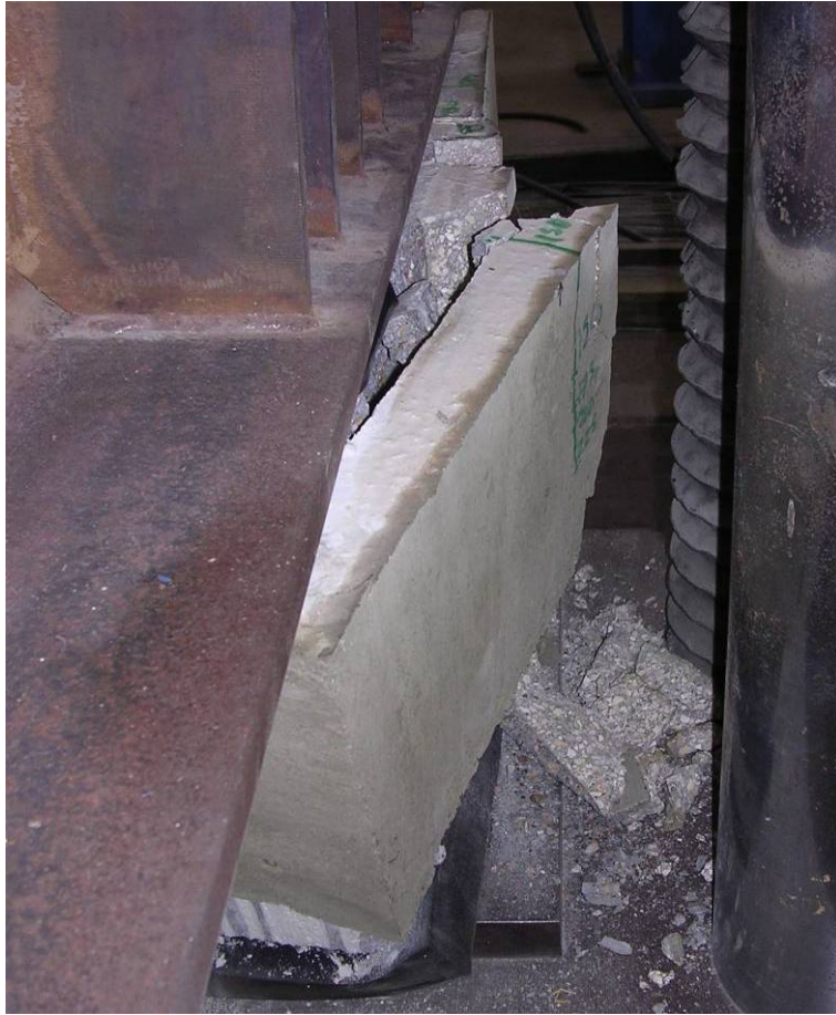
Figure 7.101: Concrete Jacket #1 Specimen Failure
