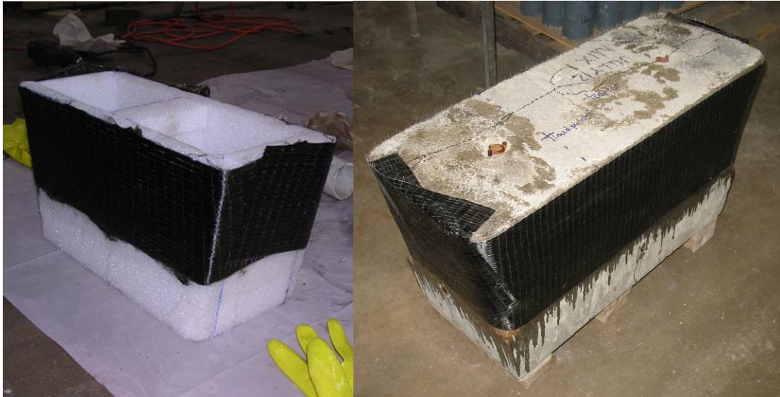
Figure 4.27: Mock-up of Specimen (Left), FRP Repaired Specimen (Right)
