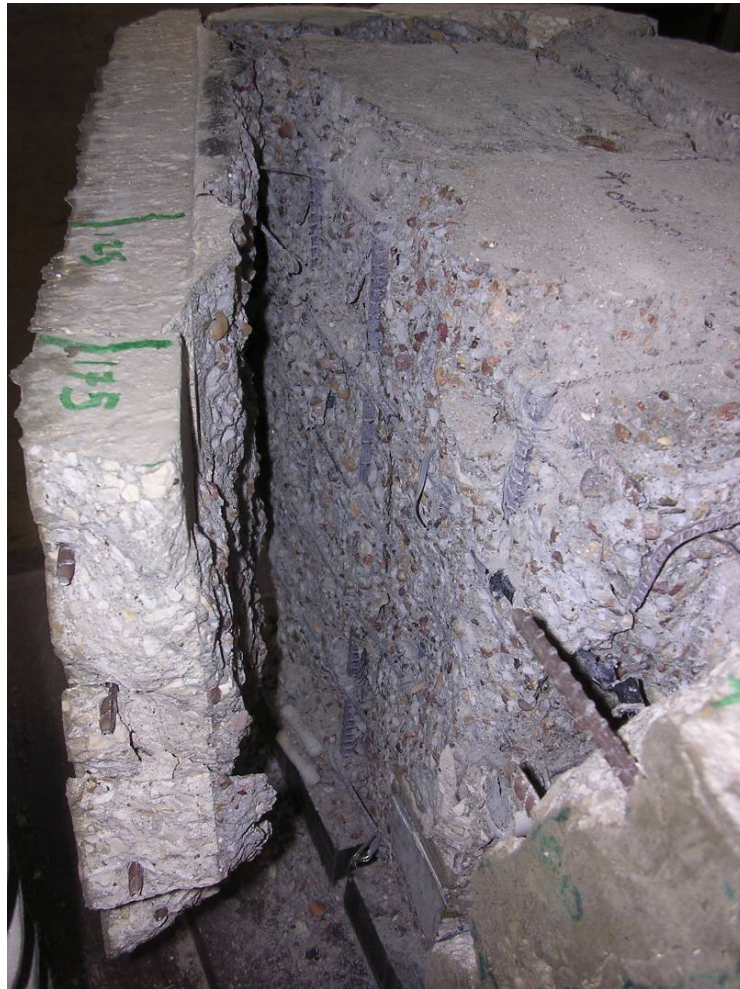
Figure 7.111: Failure of Concrete Jacket #2 Specimen
