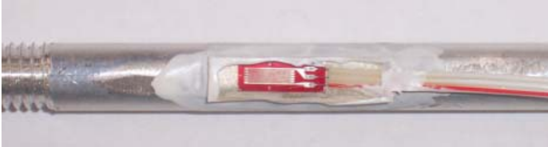
Figure A.10: Fourth, Paint with Gagekote (Barrier B)
