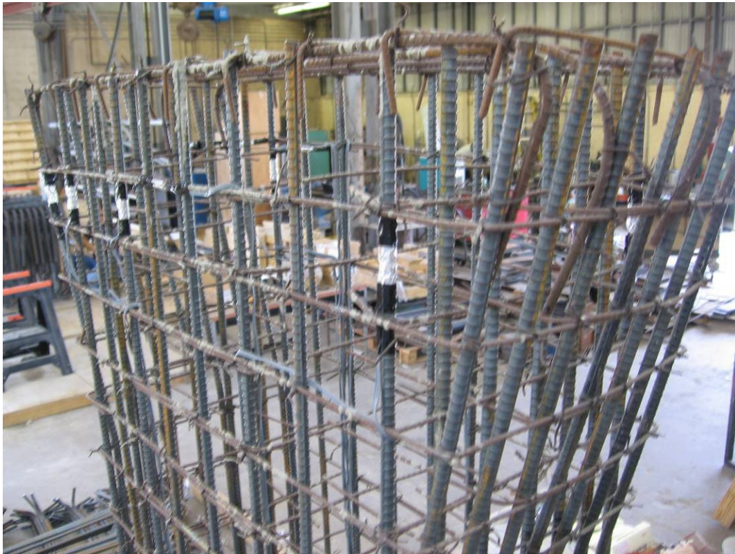
Figure 3.15: Strain Gauges of Upper Layer (Covered in Protective Foil Tape)
