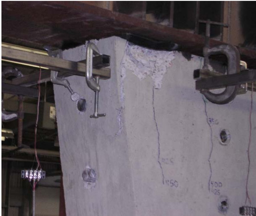
Figure 5.28: Laboratory Failure of Control Column
