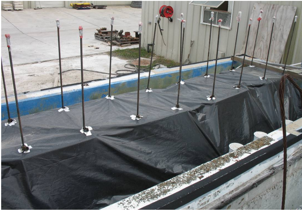
Figure 4.12: Black Plastic Covering Specimens
