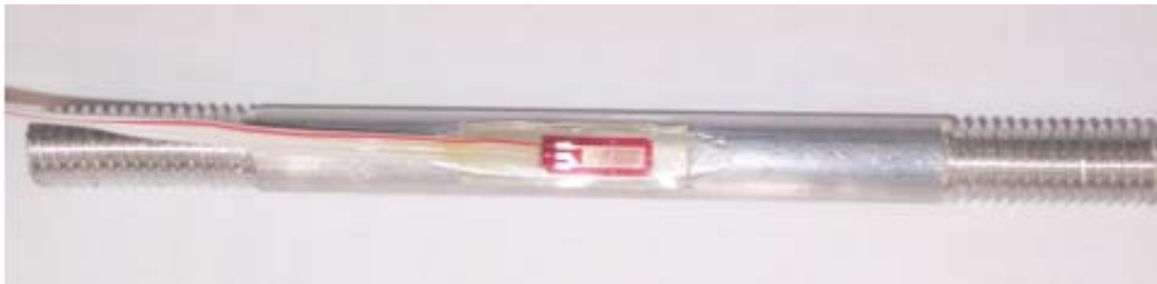
Figure A.9: Third, Apply Strain Gauge to Center
