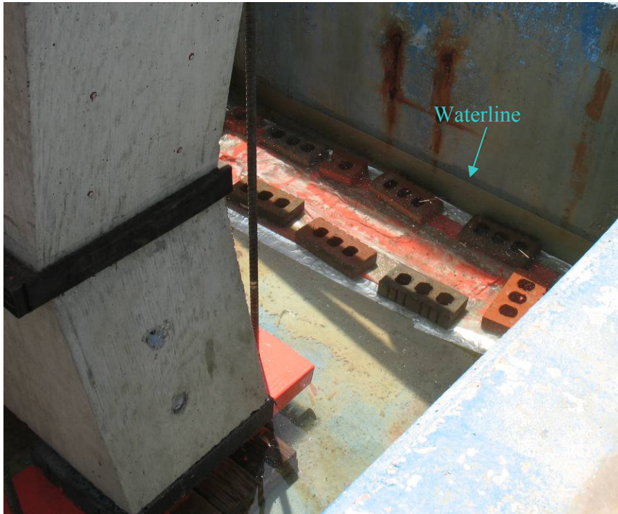
Figure 4.11: Water Flooding the Bottom of Exposure Tank
