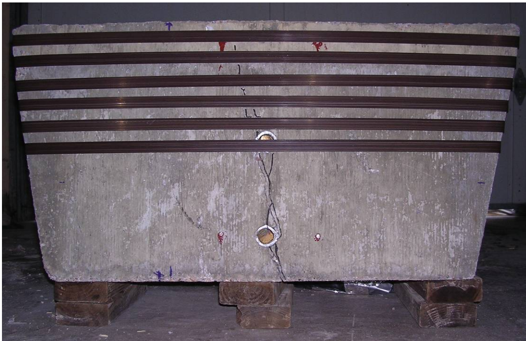
Figure 4.24: Packing Strap Repair before Testing
