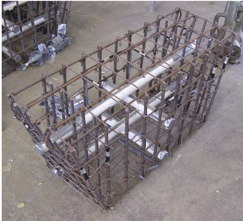
Figure 4.8: Reinforcing Cage with Strain Gauges (Covered in Protective Foil Tape)
