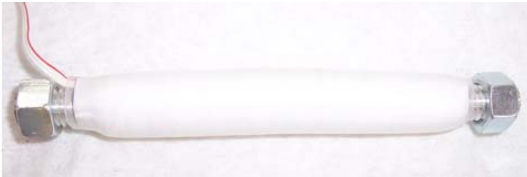
Figure A.13: Seventh, Apply Heat Shrink Tubing (4") as a Bond Breaker
