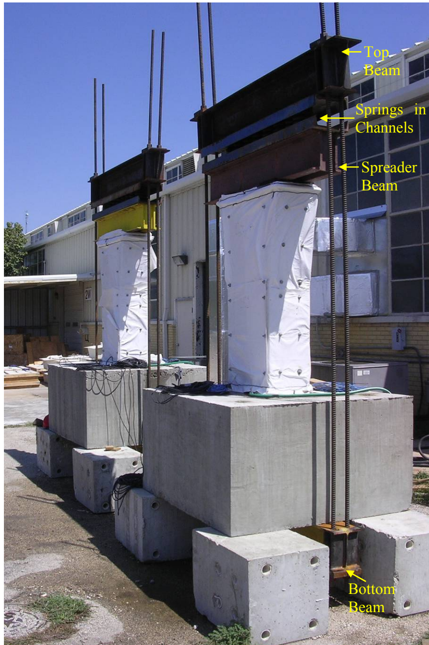
Figure 3.17: Overview of the Post-Tensioning Arrangement
