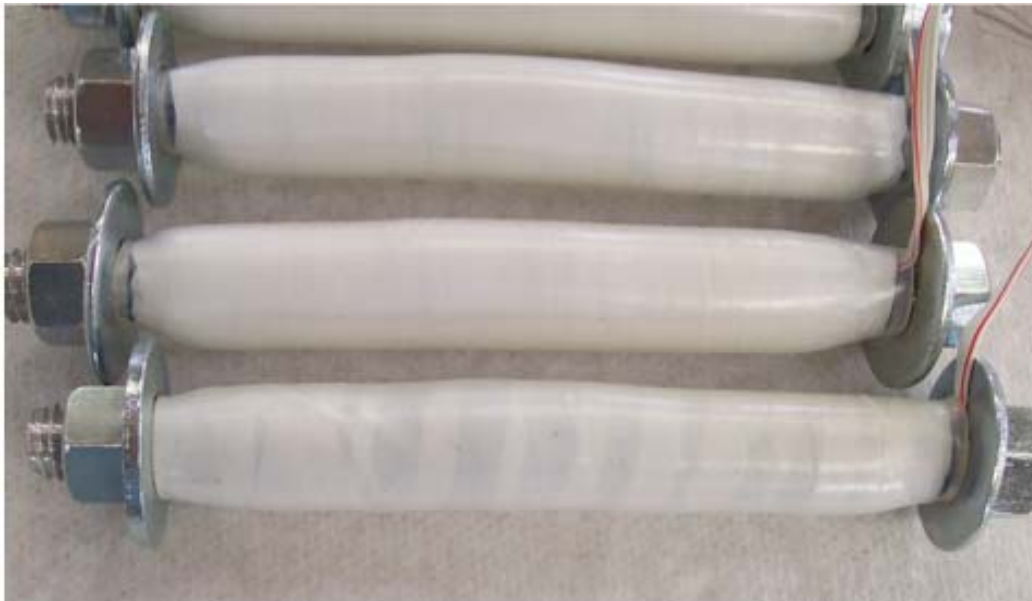
Figure A.14: Finally, Attach Washers and Set Gauge Length by Adjusting Nuts
