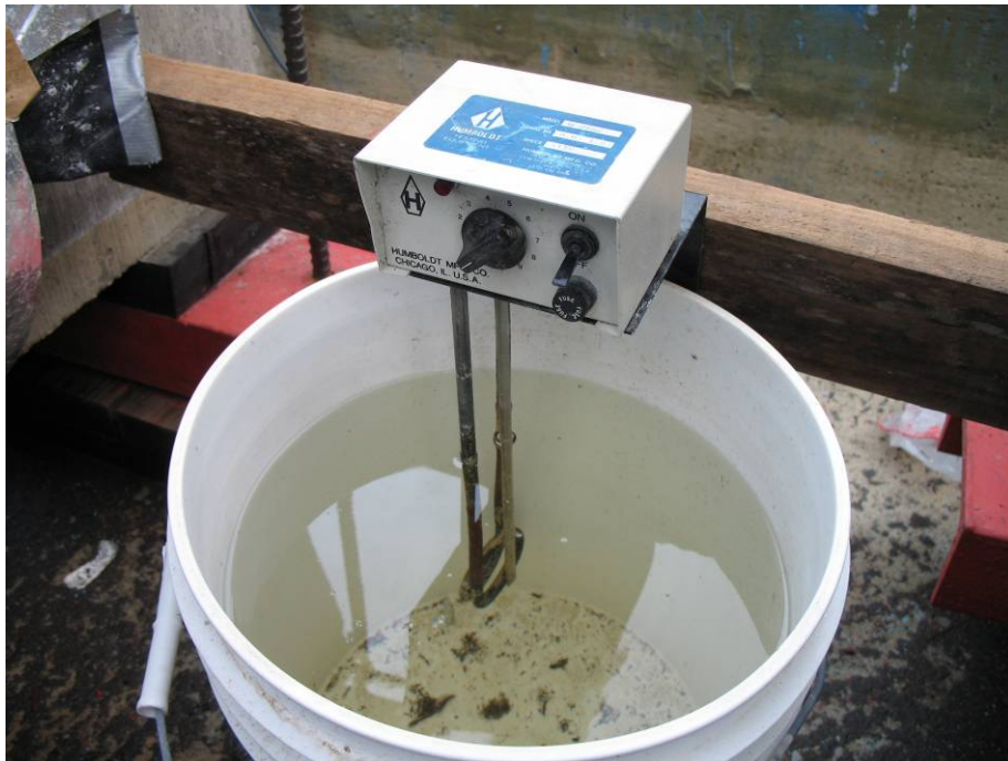
Figure 4.13: Water Heater Set-up
