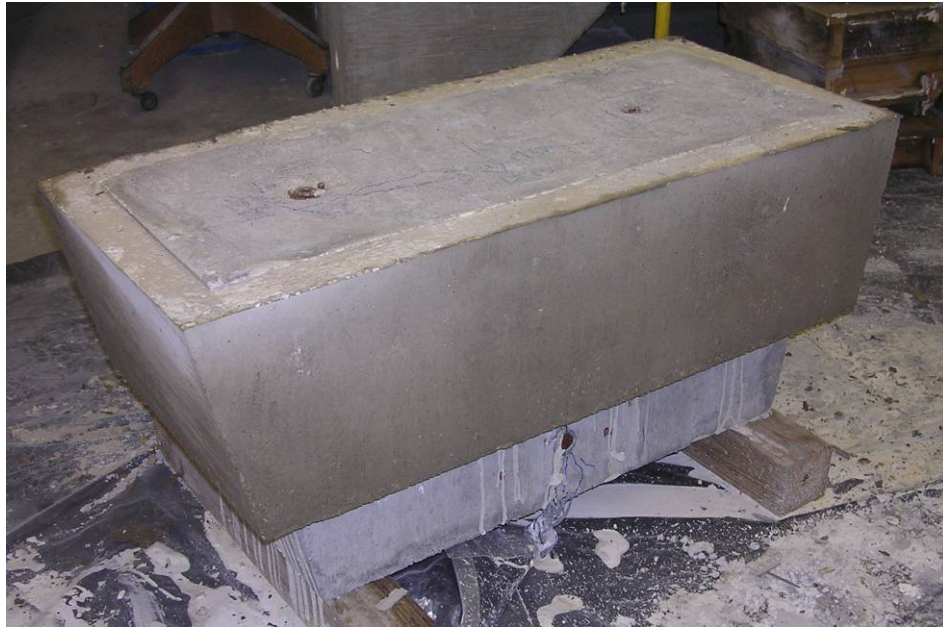
Figure 2.26: Concrete Jacket Repair on Specimen
