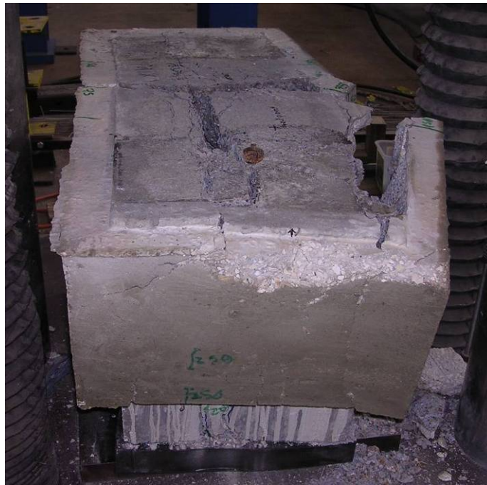
Figure 7.114: Concrete Jacket #1 Specimen Damage
