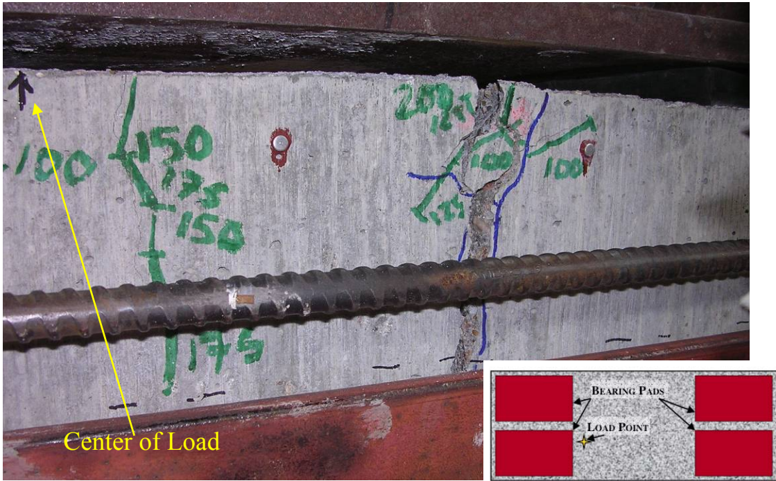
Figure 7.77: Widening of Center Crack in Post-tensioned #1 Specimen
