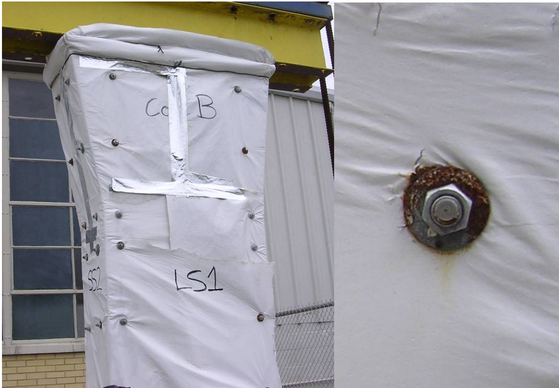
Figure 3.16: Demec Points on Column (Left) and Close-up of Demec Point (Right)
