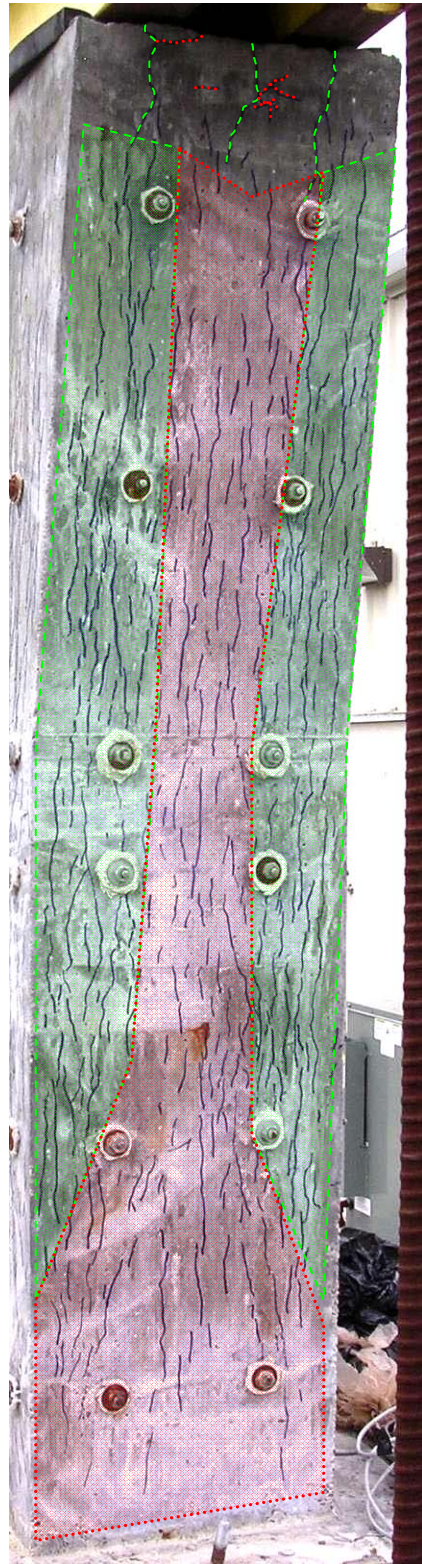
Figure 6.39: Column B South Face April 2008 (cracks marked in blue)
