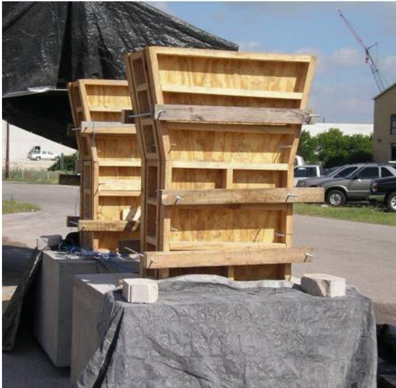
Figure 3.7: Formwork Set Up for ASR/DEF Columns 96
