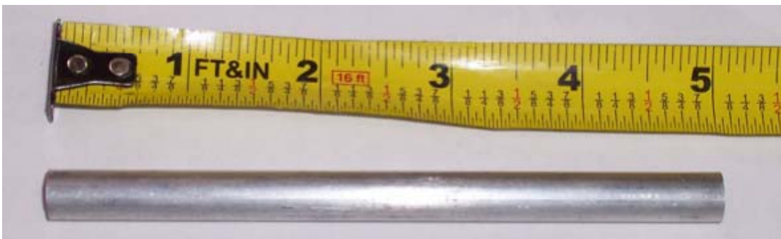
Figure A.7: First, Cut Five Inches of Aluminum Bar Stock
