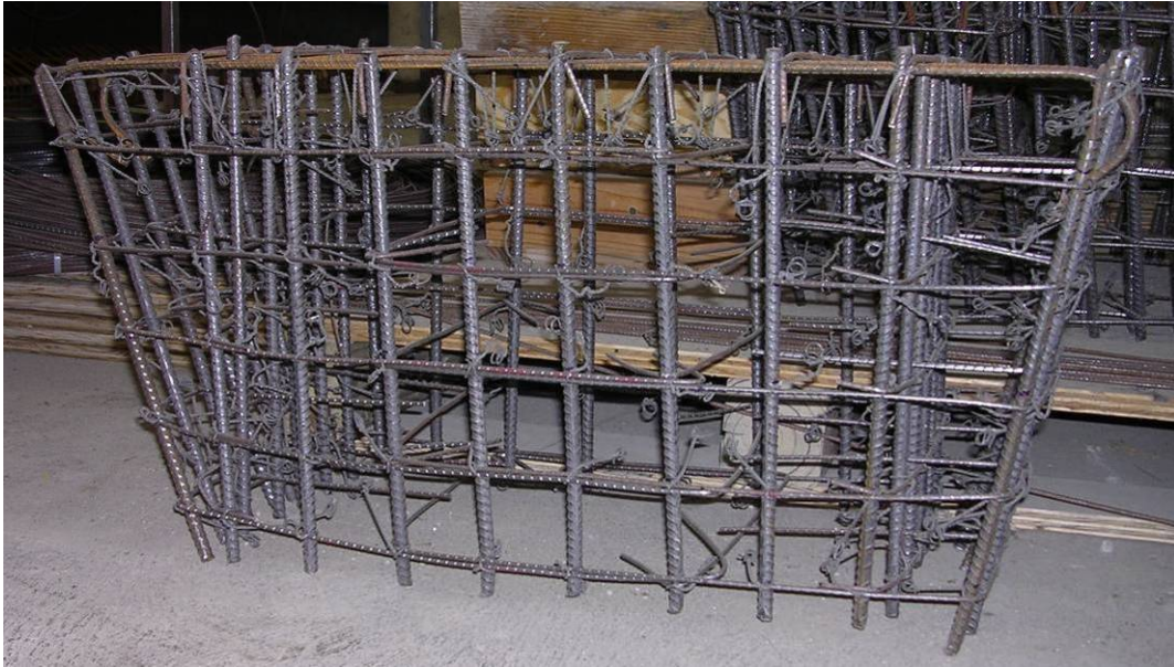
Figure 4.1: Reinforcing Cage of Bearing Specimen
